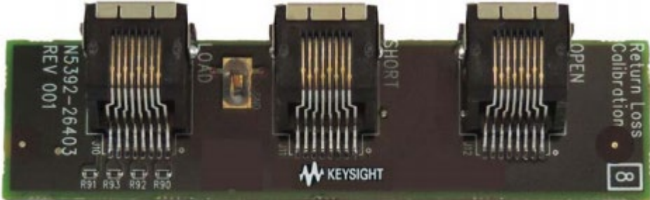
Figure 8. The return loss fixture is used to calibrate the VNA for return loss measurements and is included in the standard Ethernet fixture kit.
