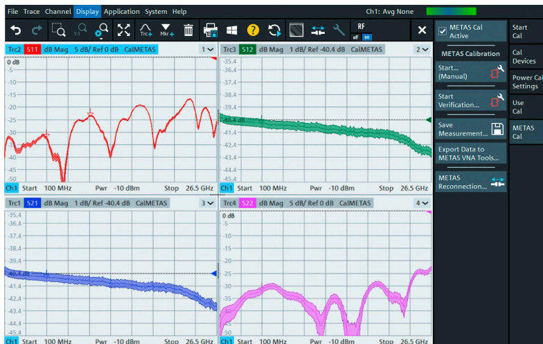
Real-time S-parameter measurements with uncertainty bands
