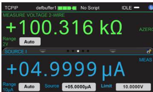
Figure 66: Resistance measurement SIMV and read ohms
