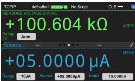
Figure 65: Resistance measurement SIMV SCPI example
