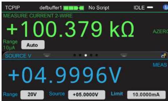
Figure 64: Resistance measurement SVMI and reading ohms
