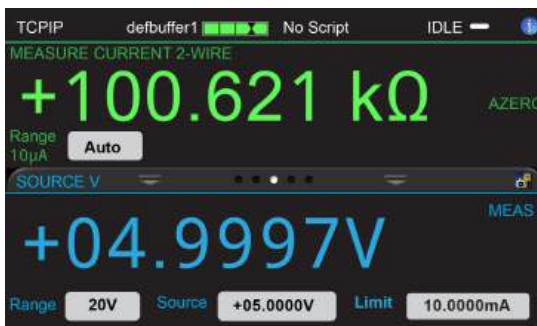
Figure 63: Resistance measurement using SVM1 and reading ohms
