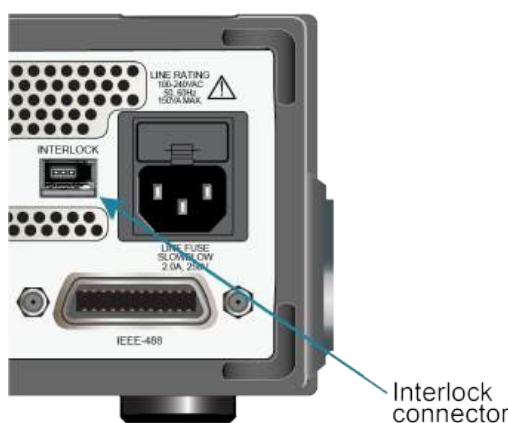
Figure 55: Rear-panel interlock location
