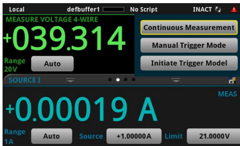
Figure 37: Measurement method indicator
