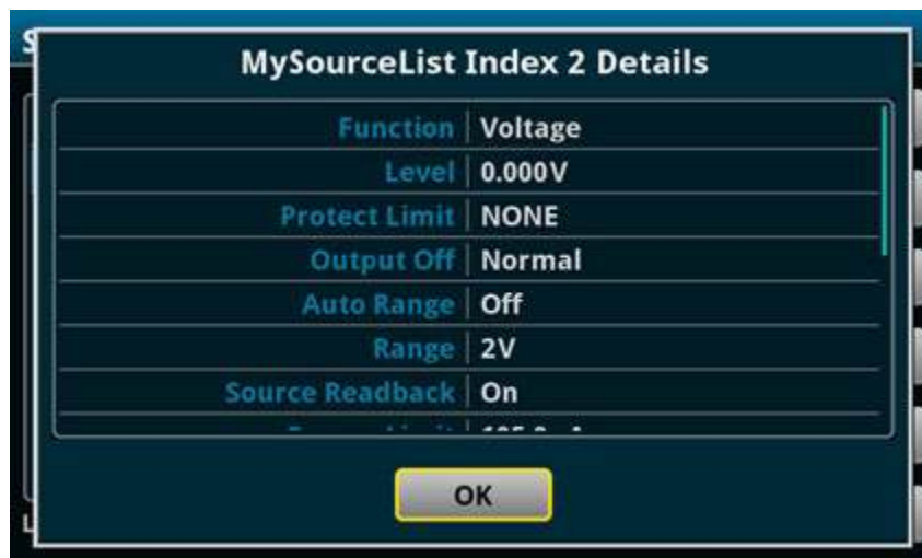
Figure 79: Source configuration list index details
