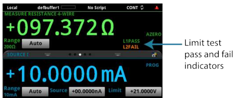
Figure 74: Limit test front-panel indicators
