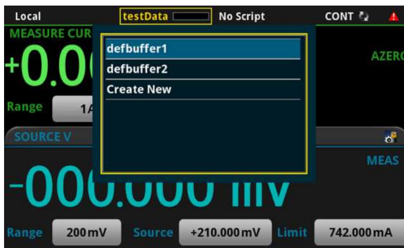
Figure 166: 2450 active buffer indicator expanded
