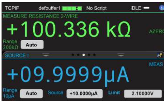
Figure 68: Resistance measurement with automatic settings
