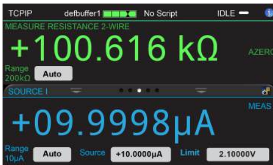
Figure 67: Resistance measurement using resistance function
