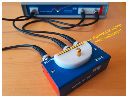
Figure 4-3: Reference plane after Open / Short / Load calibration
