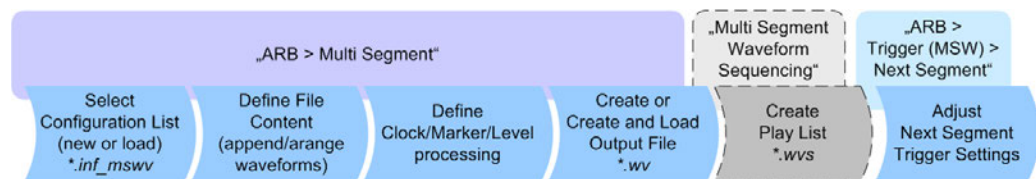
Figure 4-27: Basic workflow for generation of multi-segment waveforms
