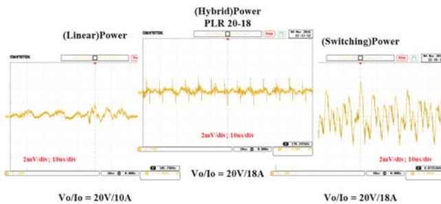
Ripple Comparison for Rating Power Output (Bandwidth : 1MHz)
