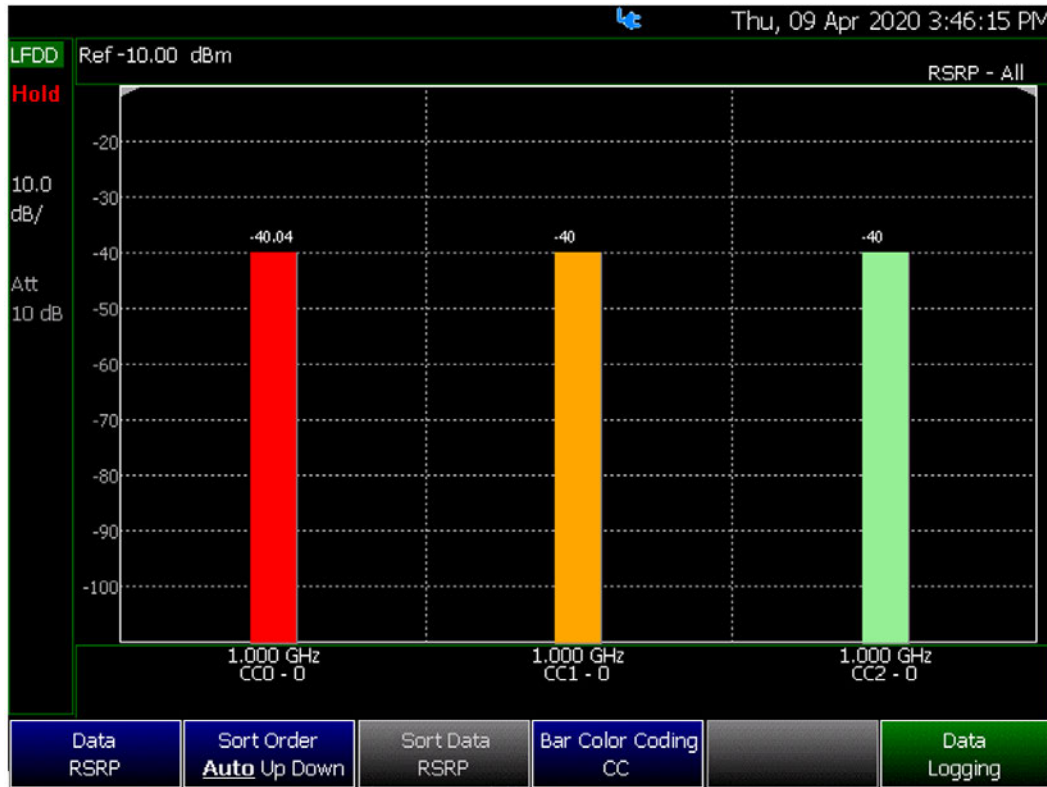
Figure 13-3 LTE FDD Bar Chart – PCC Example
