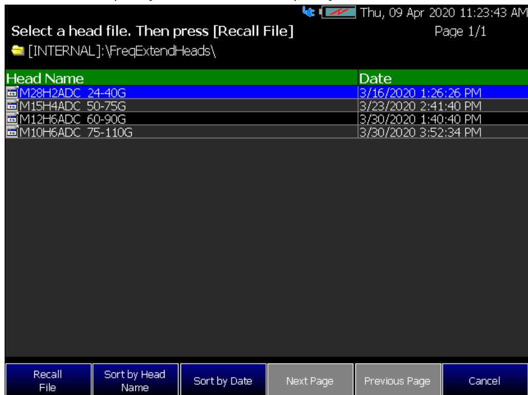
Figure 31-3 FieldFox Frequency Extender Select Frequency Extender Head
