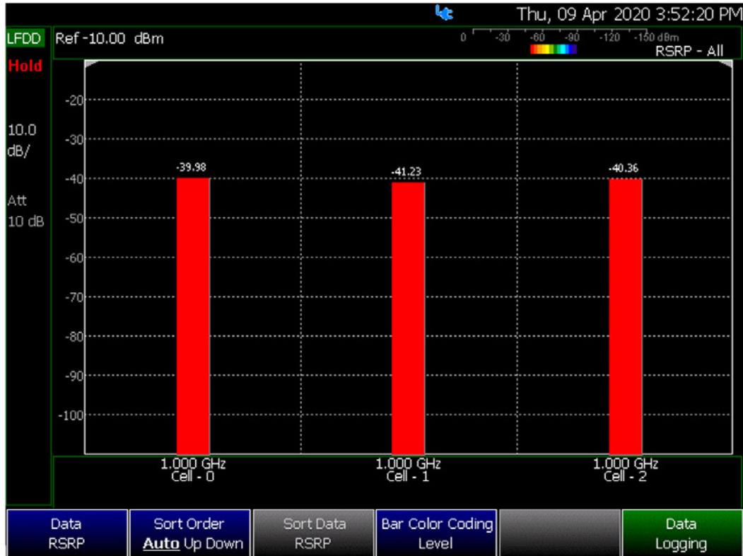
Figure 13-4 LTE FDD Bar Chart – Level Example
