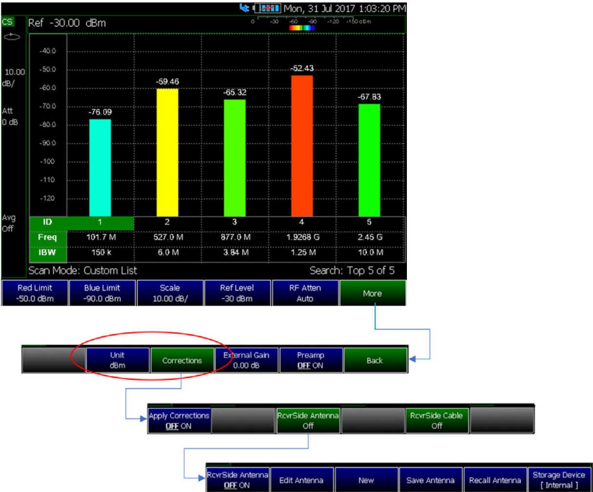
Figure 28-15 Overview of Field Strength for Channel Scanner (See also, Figure 28-16 on page 665 .)
