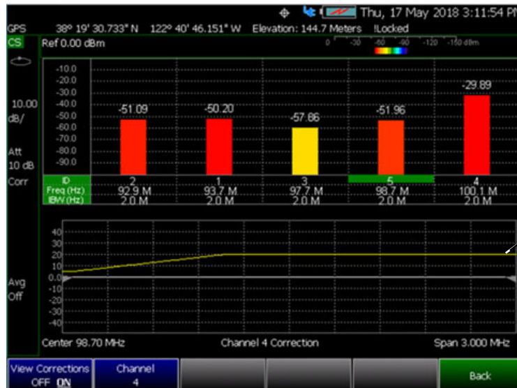
Figure 28-17 Yellow Trace with Cable and Antenna Corrections
