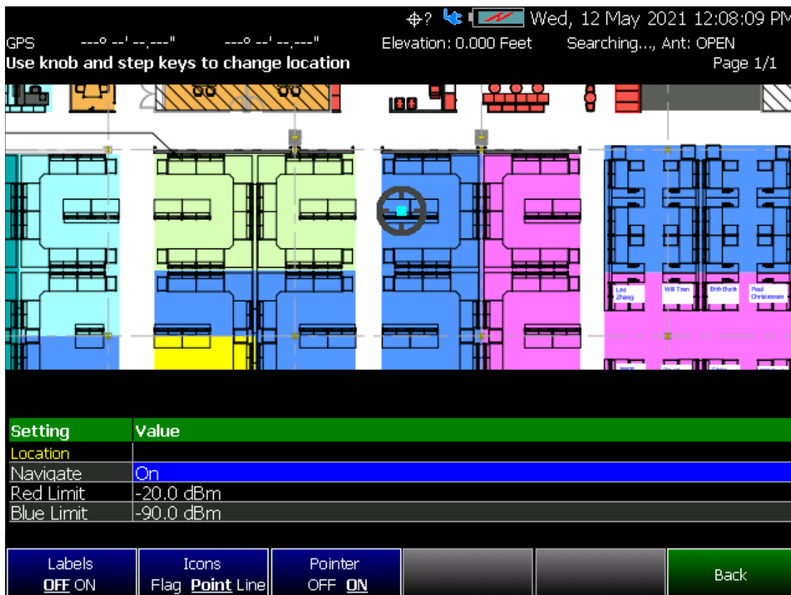
Figure 16-15 Example of an Indoor Building Map with Single Icon and Bore Sight Pointer
