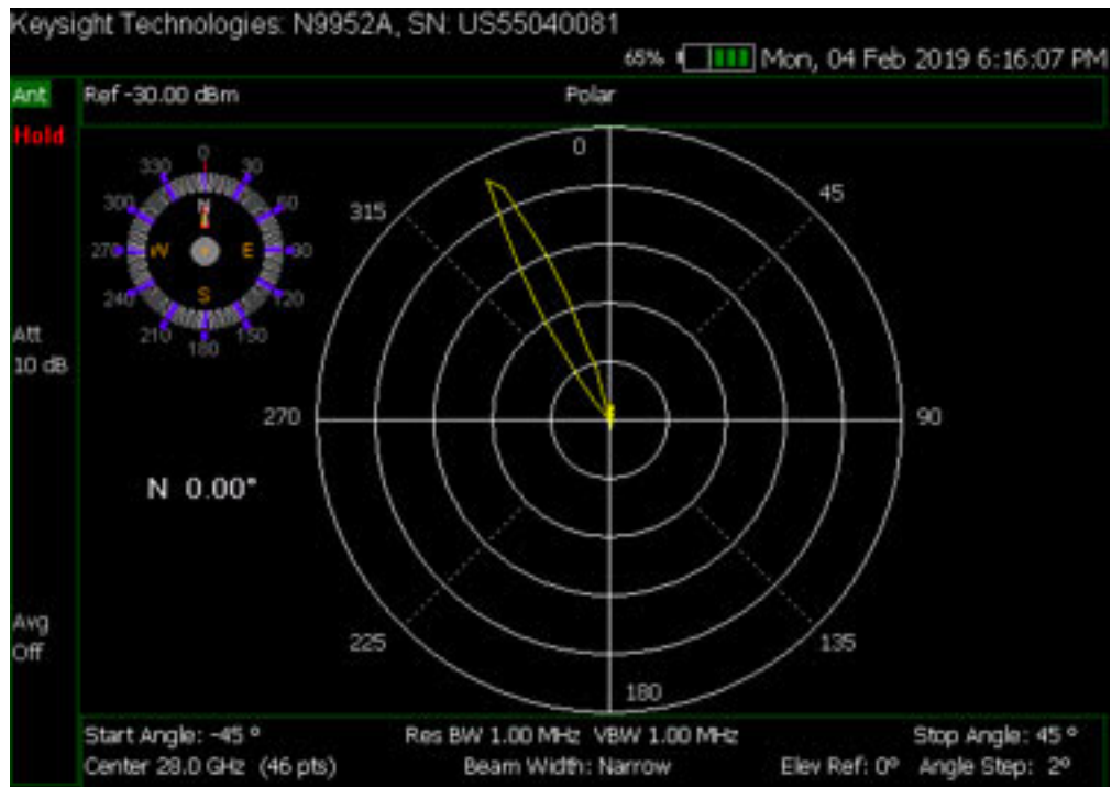
Figure 14-3 Polar Scan with compass displayed
