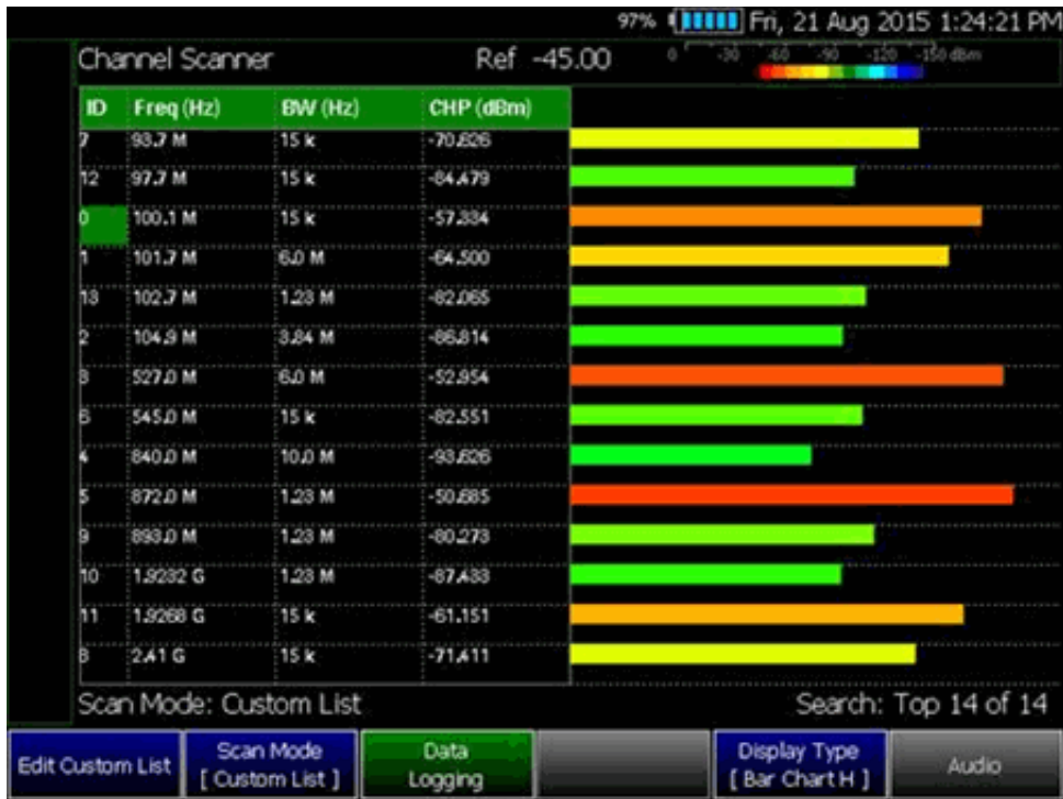
Figure 28-6 Bar Chart Horizontal Display Type
