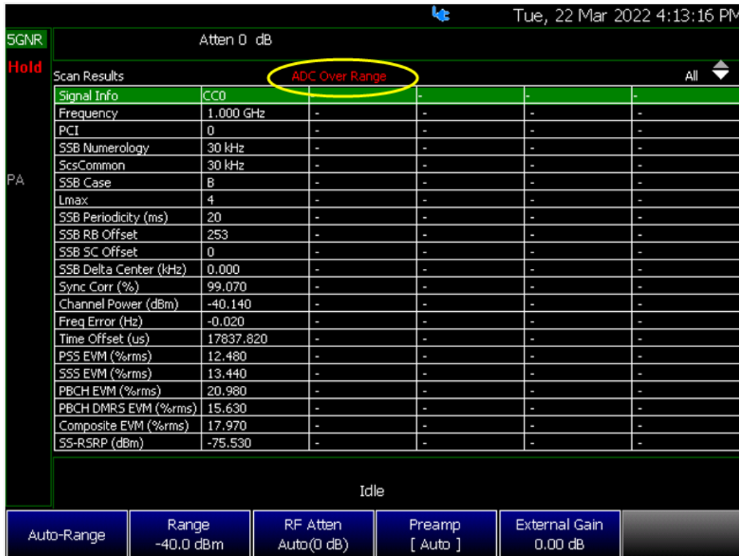
Figure 13-33 OTA 5G NR Signal Before Auto-Range – Table
