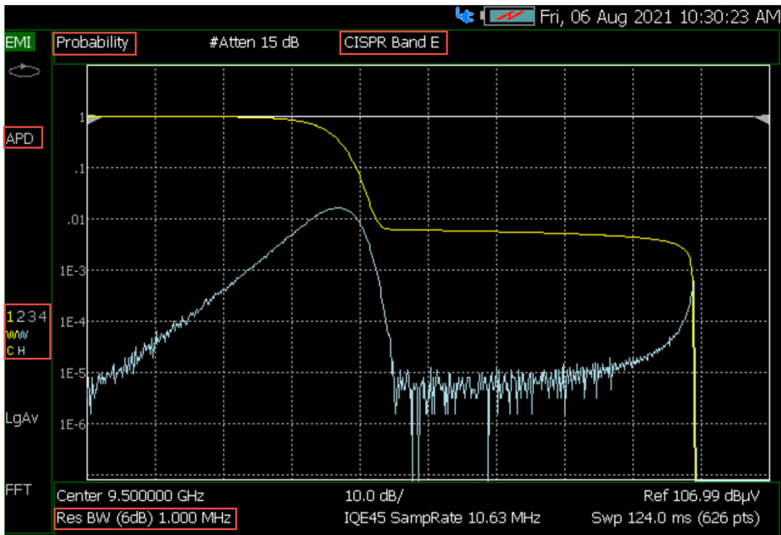
Figure 12-5 APD Statistics Example 2 – CW
