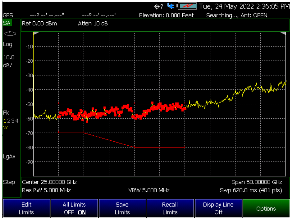
Figure 30-11 Example: Recalled Limit Line Formatting LimitExample.csv
