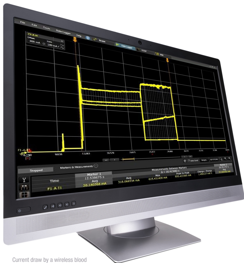
Current draw by a wireless blood pressure monitor
