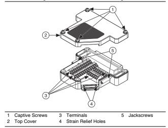
Figure 2. NI 9923 Parts Locator Diagram
