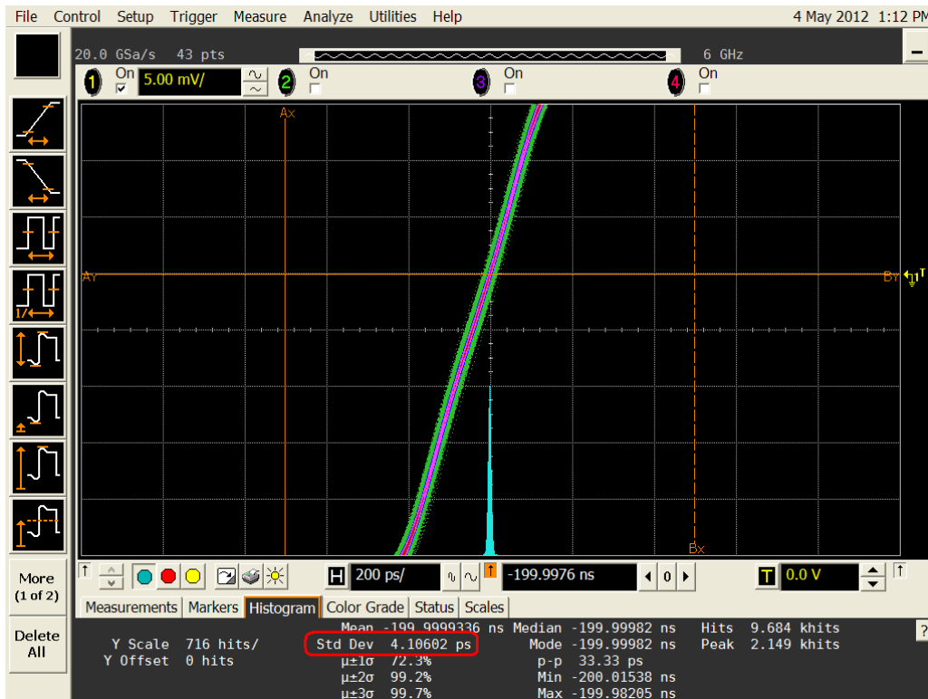
Figure 3. Jitter measurement on Trueform signal.
