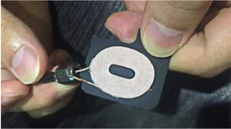
Figure 4. Transmit-receive coils in the spinal cord stimulation implant
