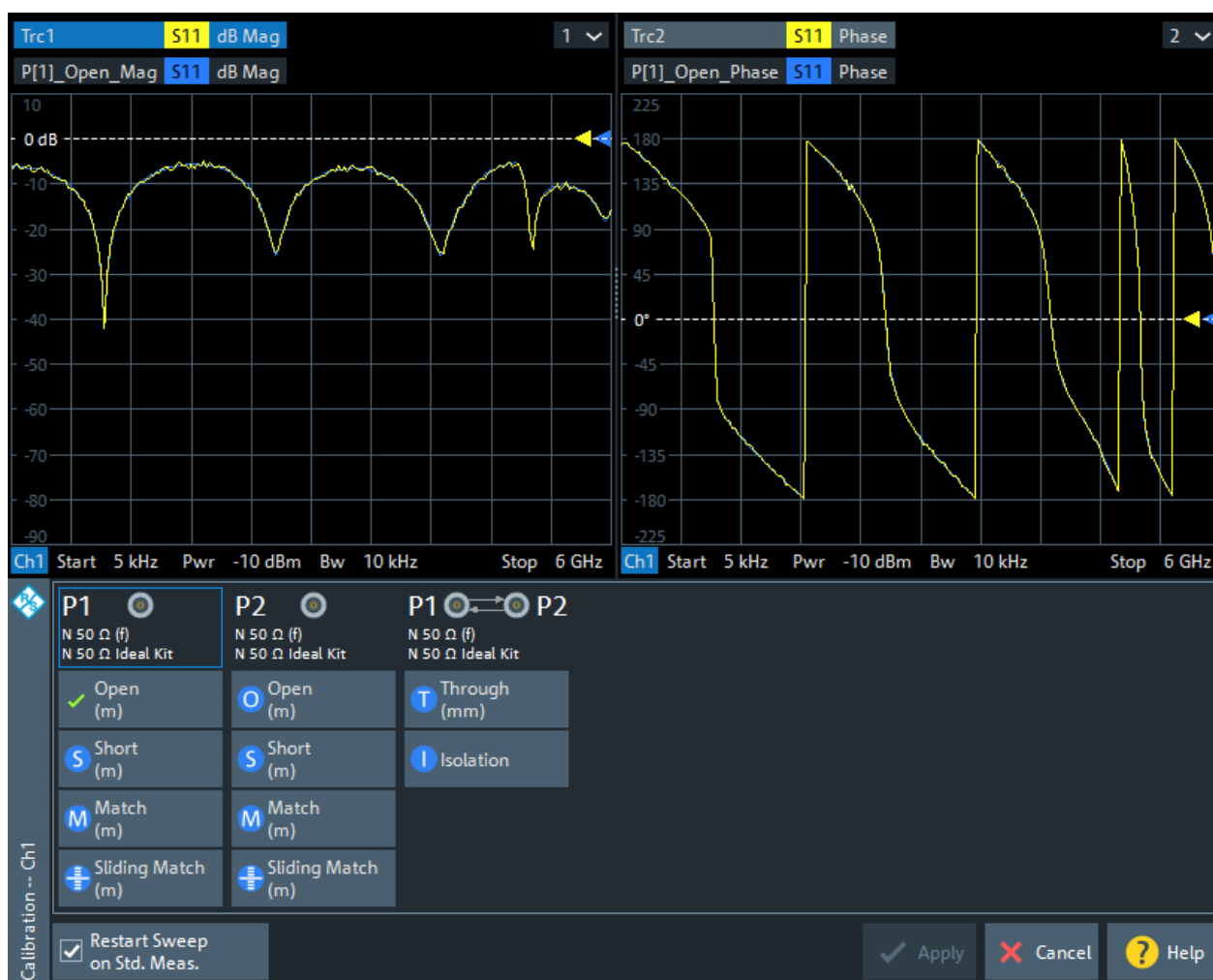
Figure 10-18: Calibration Setting Wizard, Step 3: Calibration
