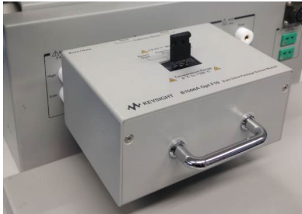
Figure 2. The inline package socket module
