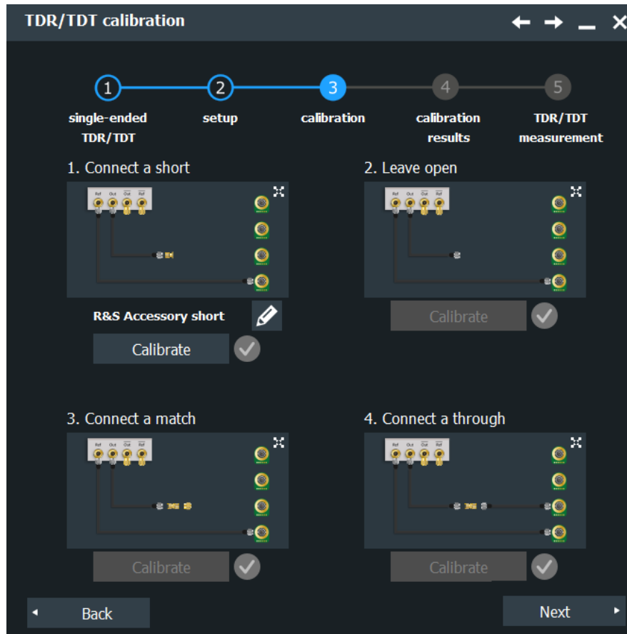
Figure 16-5: Calibration of differential TDR/TDT
