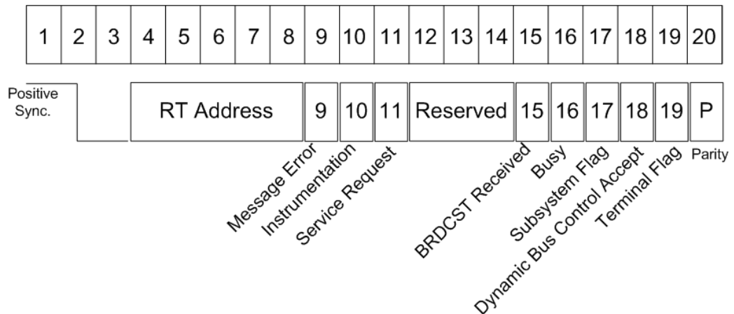
Figure 13-12: Structure of a status word
