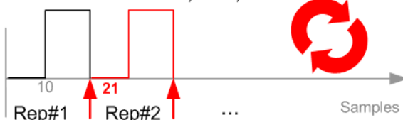
Figure 4-21: Example: Processing of MARKER TRACE if CONTROL LENGTH is not used
