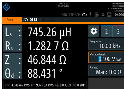
Primary inductance measurement at 10 kHz and 100 mV (RMS)
