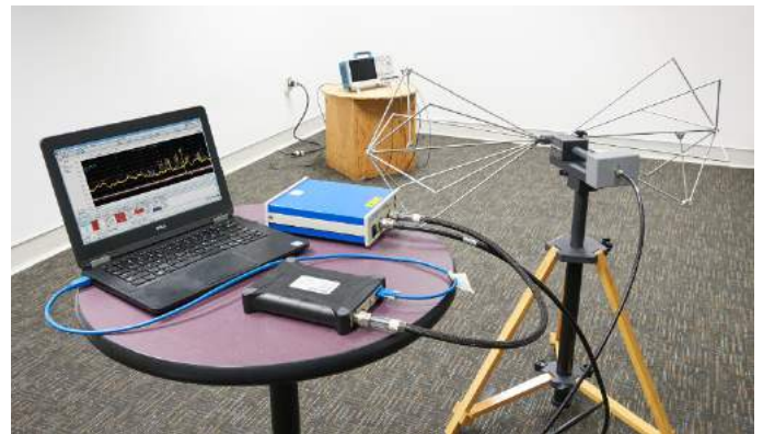
FIGURE 13. A typical pre-compliance test setup in a large room. The spacing between the EMI antenna and equipment under test is 3m.
