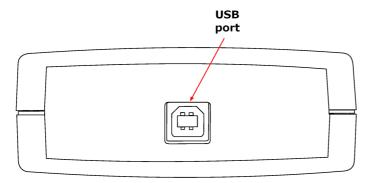
**USB port:** use the USB cable supplied to connect this to the PC that is running the Pico software. A PC with a USB 2.0 port or faster is recommended for best performance.
