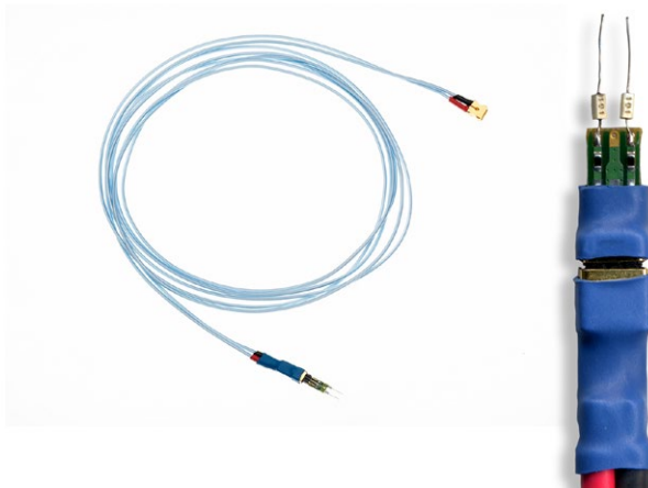
TriMode™ High-temperature Tip: When used with the 1.5 m Socket Cable XL, this tip can be used in environments from –55 °C to 150 °C. Up to 10 GHz bandwidth with DSP.
