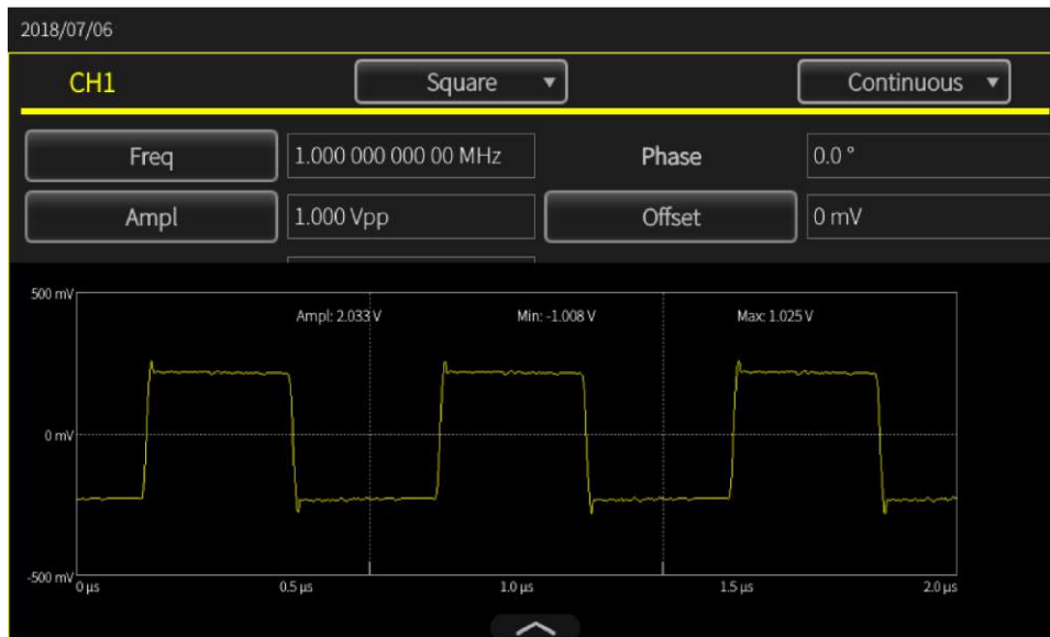
Figure 71: CH1 oscilloscope 1 MΩ - InstaView
