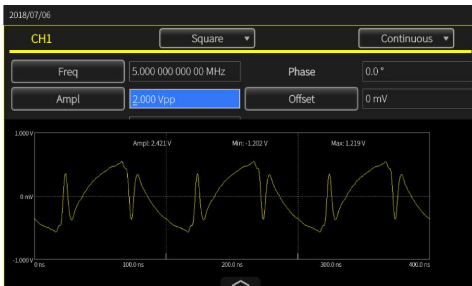
Figure 73: Frequency 5 MHz - scope
