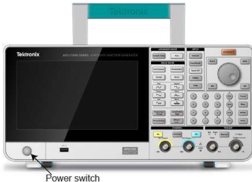
Figure 18: AFG31000 Series two-channel front view
