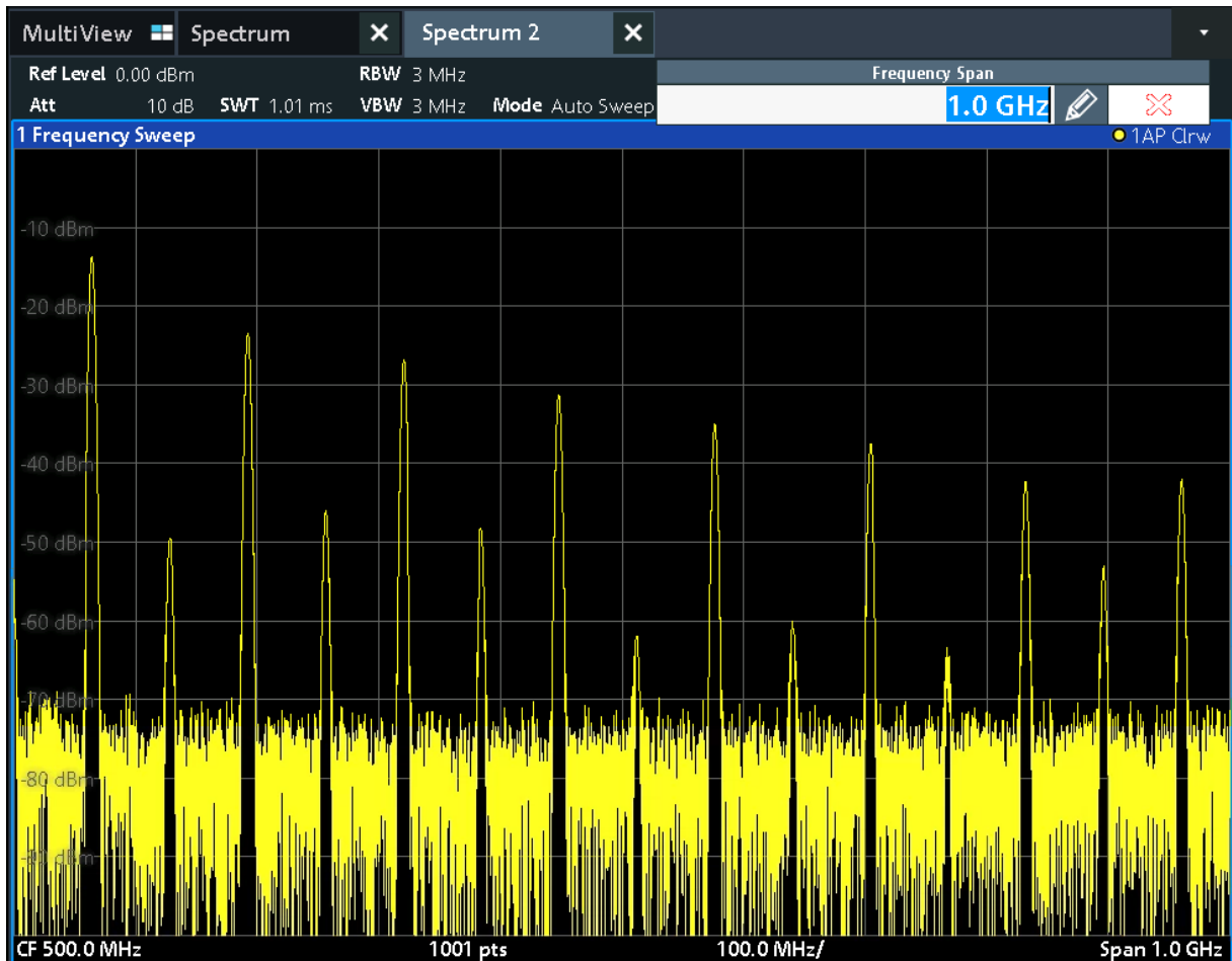
Figure 6-6: Frequency spectrum of the calibration signal with a larger span
