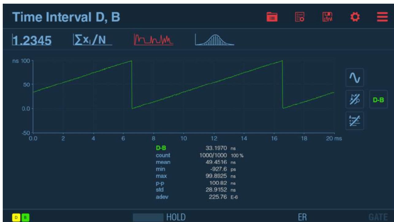
Fig. 5.6: Time Interval Continuous of 2 clock signals with constant frequency offset
