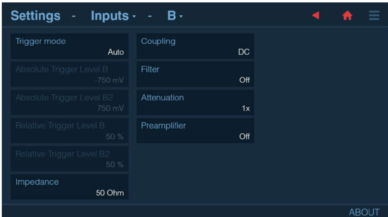
Fig. 5.12: Example configuration for Time Interval A to A to B to B measurement
