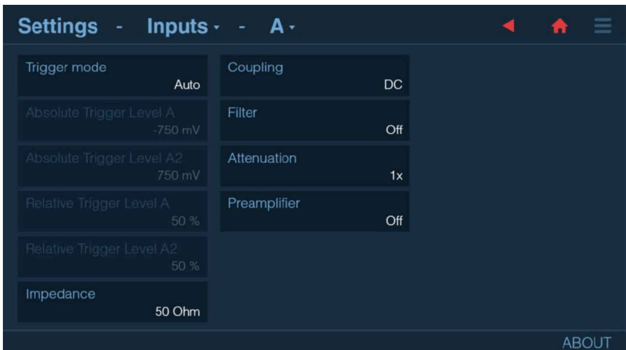
Fig. 5.11: Example configuration for Time Interval A to A to B to B measurement
