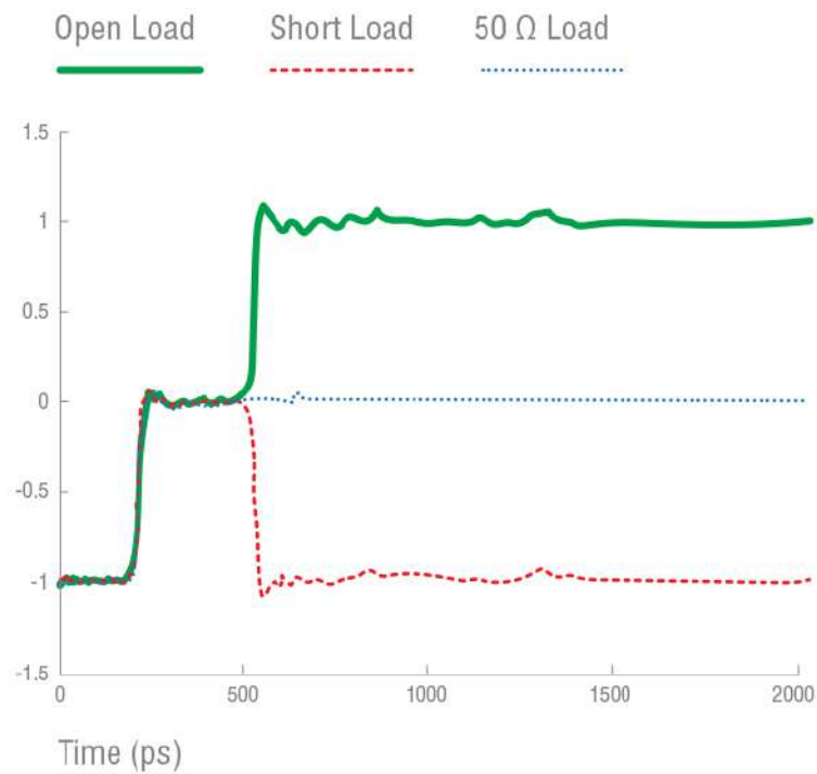
Fig. 5.8: Measuring Time Interval between 2 levels of reflected signal in TDR measurement allows to calculate the distance to cable break
