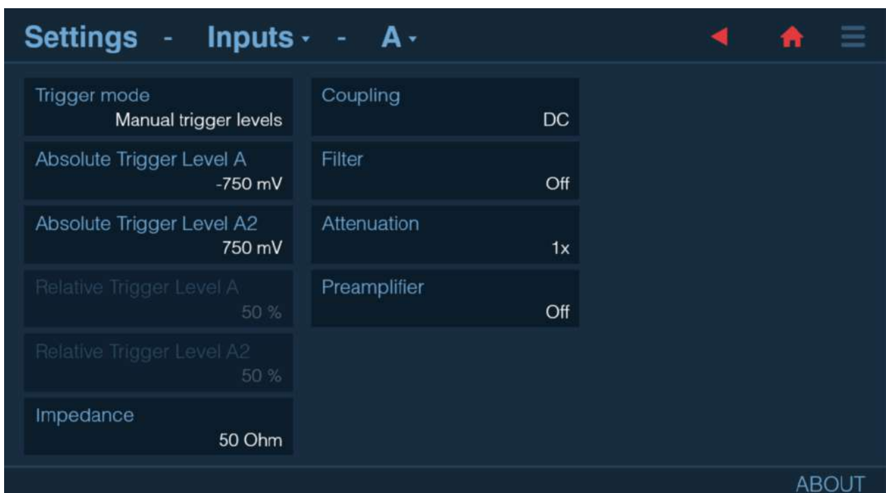
Fig. 5.9: Instrument's configuration for TDR measurement on Figure 28
