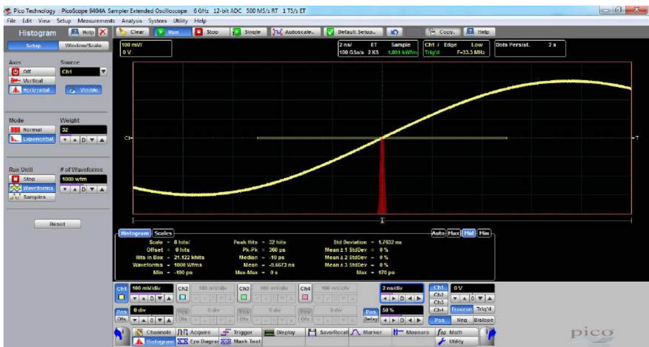
An example of the horizontal histogram display
