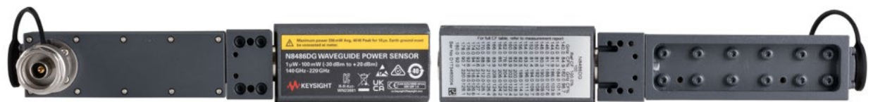
Figure 7. N8486DG-100 comes without built-in EEPROM with a dynamic range of -30 to +20 dBm. Users need to pre-enter calibration factors printed on the back of the sensor into the power meter.
