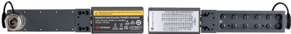
Figure 5. N8486DD-100 comes without built-in EEPROM with a dynamic range of -30 to +20 dBm. Users need to pre-enter calibration factors printed on the back of the sensor into the power meter.
