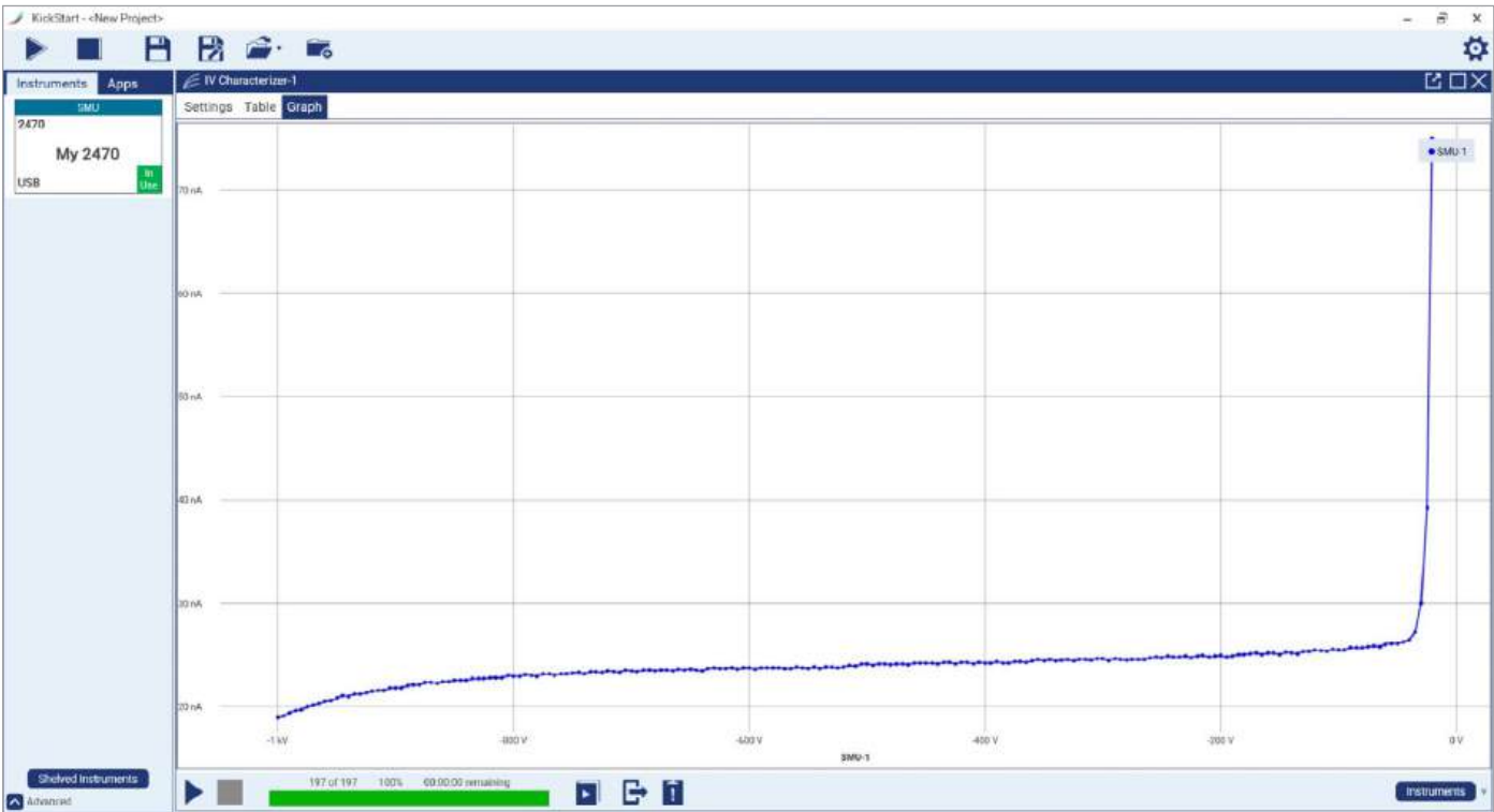
Figure 9: Leakage current results of High Voltage Diode using 2470 and KickStart
