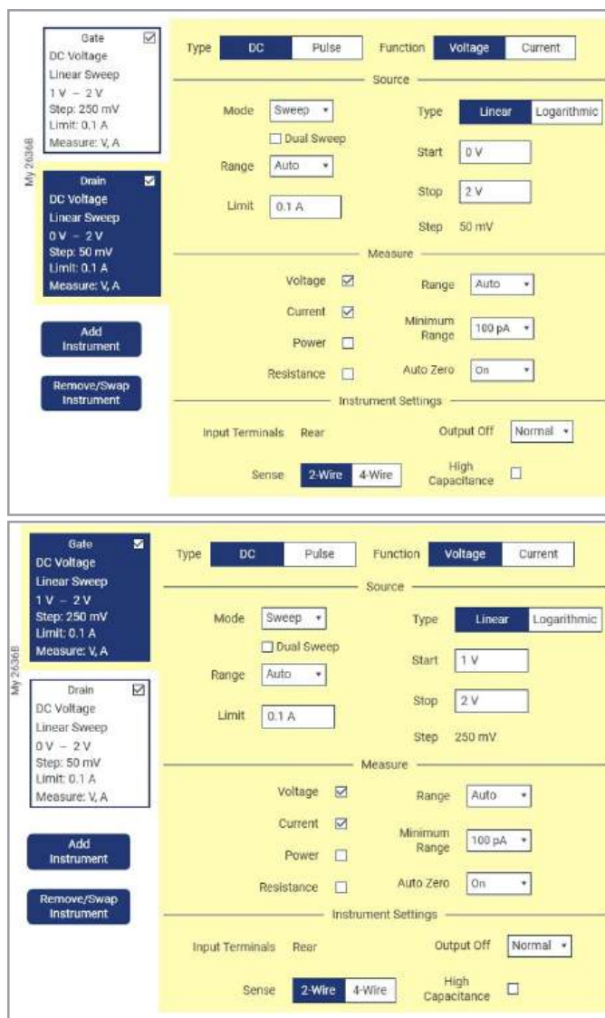
Figure 8. Drain (top) and gate (bottom) settings for output measurement in KickStart.
