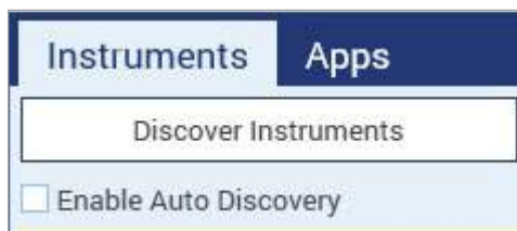
Figure 10: The KickStart Software Instrument Auto Discovery enablement checkbox that can be accessed by pressing the F12 key while viewing the Instruments Tab.
