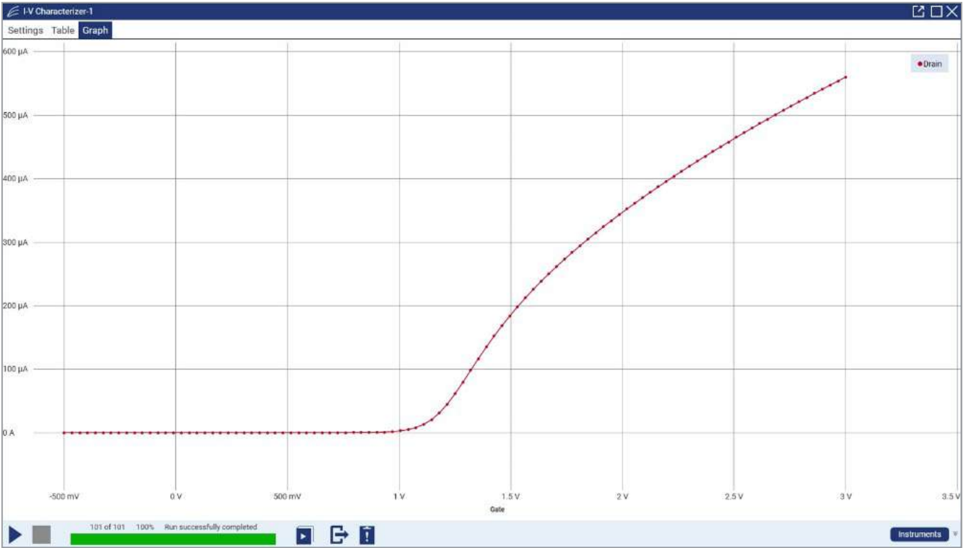
Figure 5. Transfer curve in linear scale shown in the KickStart I-V Characterizer App.
