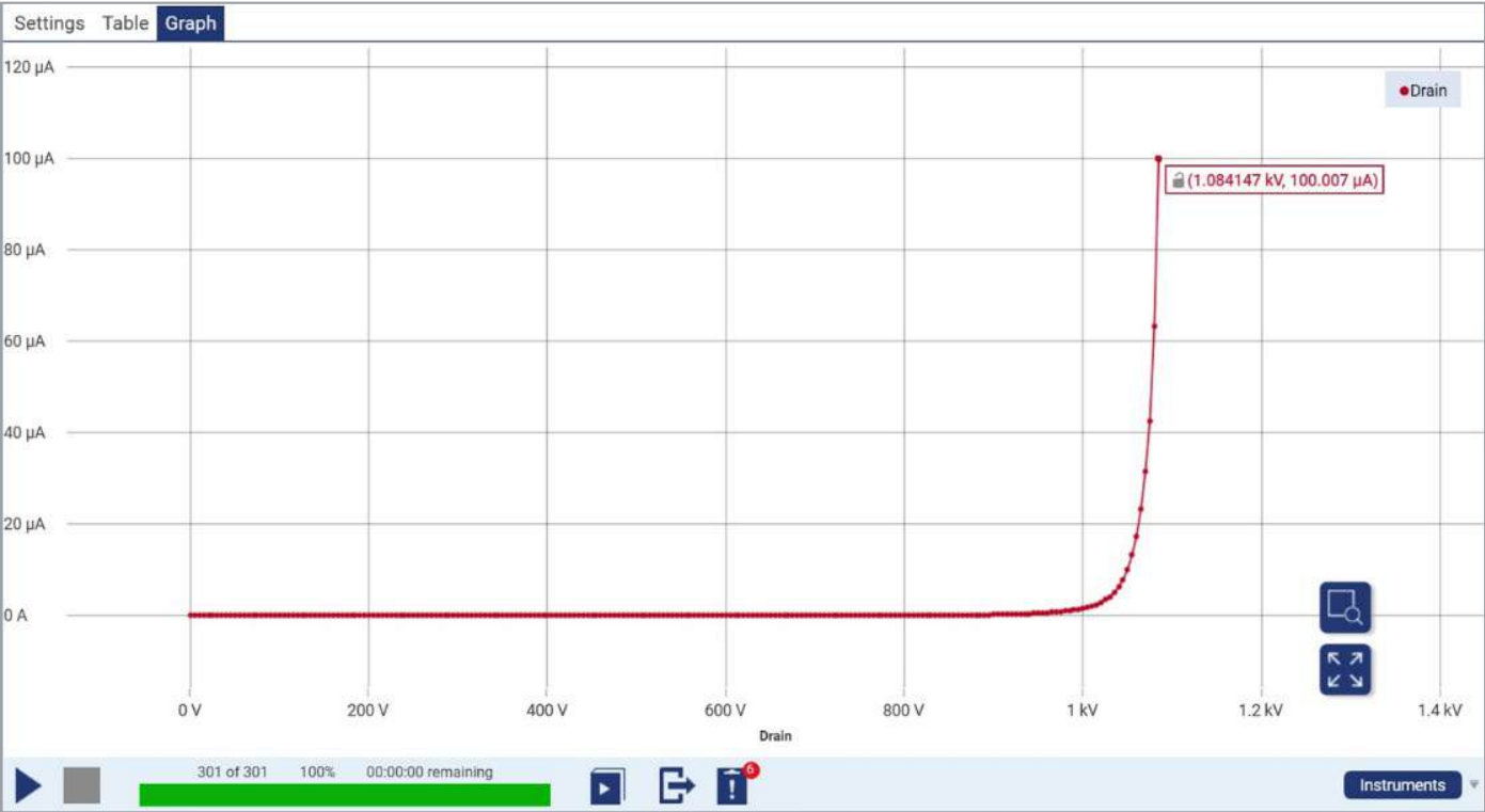
Figure 7. Breakdown Voltage (BVDSS) Test in Sweeping the Drain Voltage.
