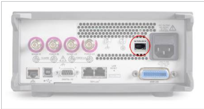
Figure 4: Location of safety interlock connection on rear panel of 2470 SMU
