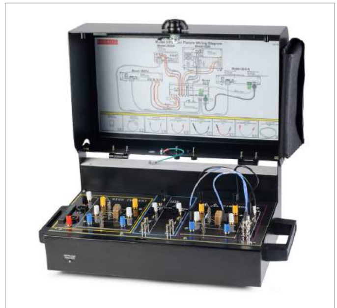
Figure 3: Properly grounded testing fixture
