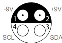
Probe's power supply pin assignment "cable view"
