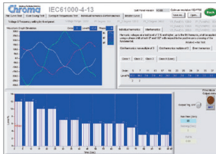
Voltage Harmonic & Interharmonic Test
