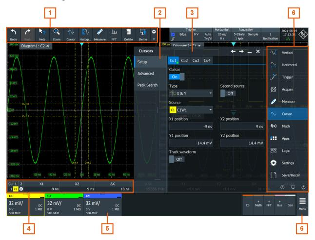
Figure 6-6: Control elements on the touchscreen
