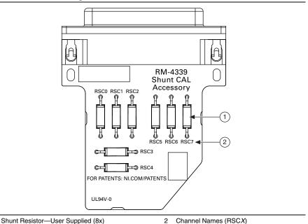
Figure 7. SCAL-4339 Resistor Locations
