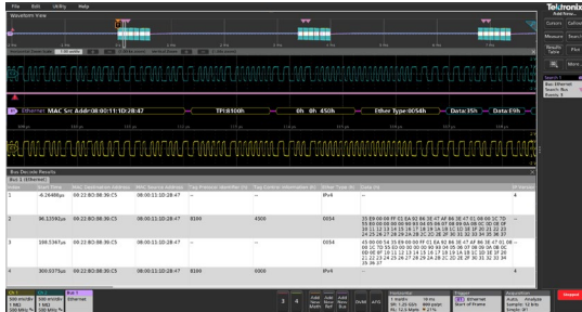
100BASE-T Ethernet decoding and triggering with results table
