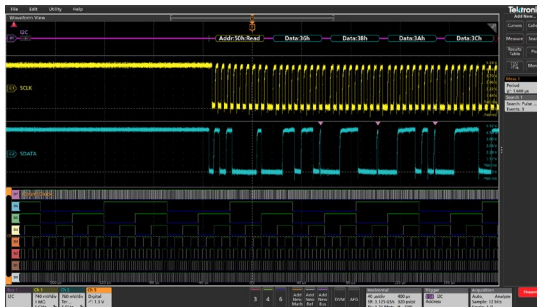
I²C decoding synchronized with digital waveforms from a TLA058 logic probe
