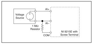
Figure 5. Connecting a Floating Differential Voltage Signal to the NI 9215E with Screw Terminal
