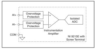
Figure 7. Input Circuitry for One Channel on the NI 9215E with Screw Terminal
