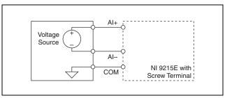
Figure 4. Connecting a Grounded Differential Voltage Signal to the NI 9215F with Screw Terminal
