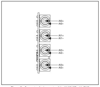
Figure 3. Connector Assignments of the NI 9215E with BNC
