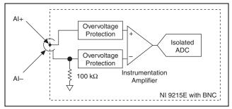
Figure 8. Input Circuitry for One Channel on the NI 9215E with BNC
