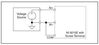
Figure 6. Connecting a Single-Ended Voltage Signal to the NI 9215F with Screw Terminal
