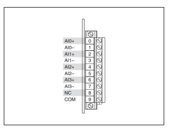
Figure 2. Terminal Assignments of the NI 9215E with Screw Terminal
