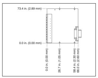
Figure 1. NI 9215E Dimensions in Millimeters (Inches)
