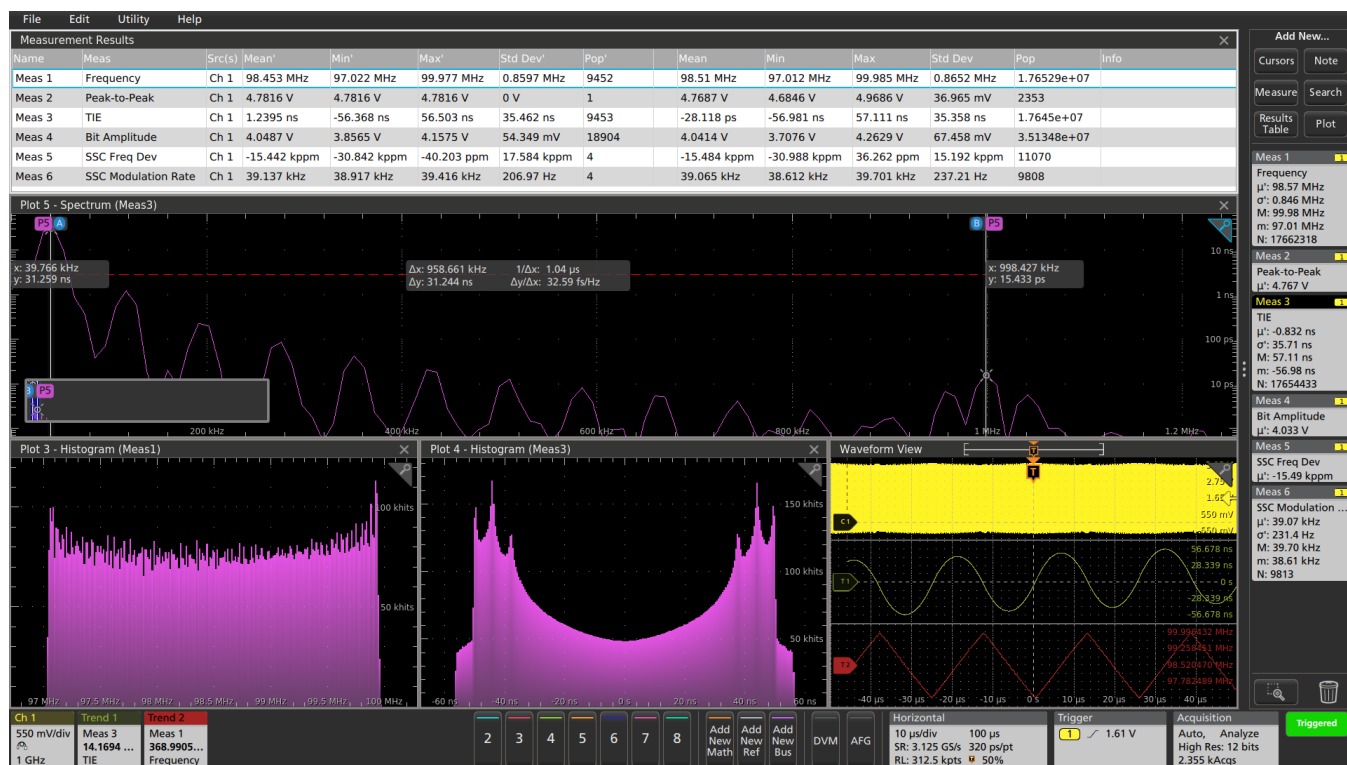
Figure 3: Analysis of a spread spectrum clock signal, showing the 39 kHz triangular modulation on the 98 MHz clock.
