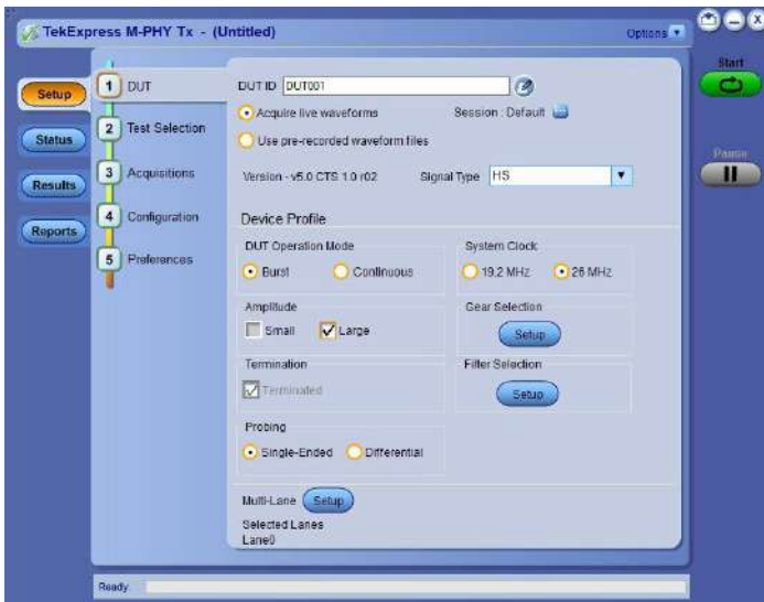
TekExpress M-PHY Tx (Options MPHY40, MPHY50) - TekExpress M-PHY Tx provides support for 100% of tests as per Spec 5.0. This solution is designed for engineers doing verification and validation as per the CTS for High Speed (HS)-Gear1, Gear2, Gear3, Gear4, and Gear5 for MPHY50 and HS-Gear1, Gear2, Gear3, and Gear4 for MPHY40. It also supports UFS4.0 reference Clock measurements in both Option MPHY50 and Option MPHY40 products.
