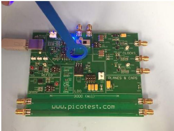
FIGURE 8. A near field probe is used to help identify potential sources of emissions.
