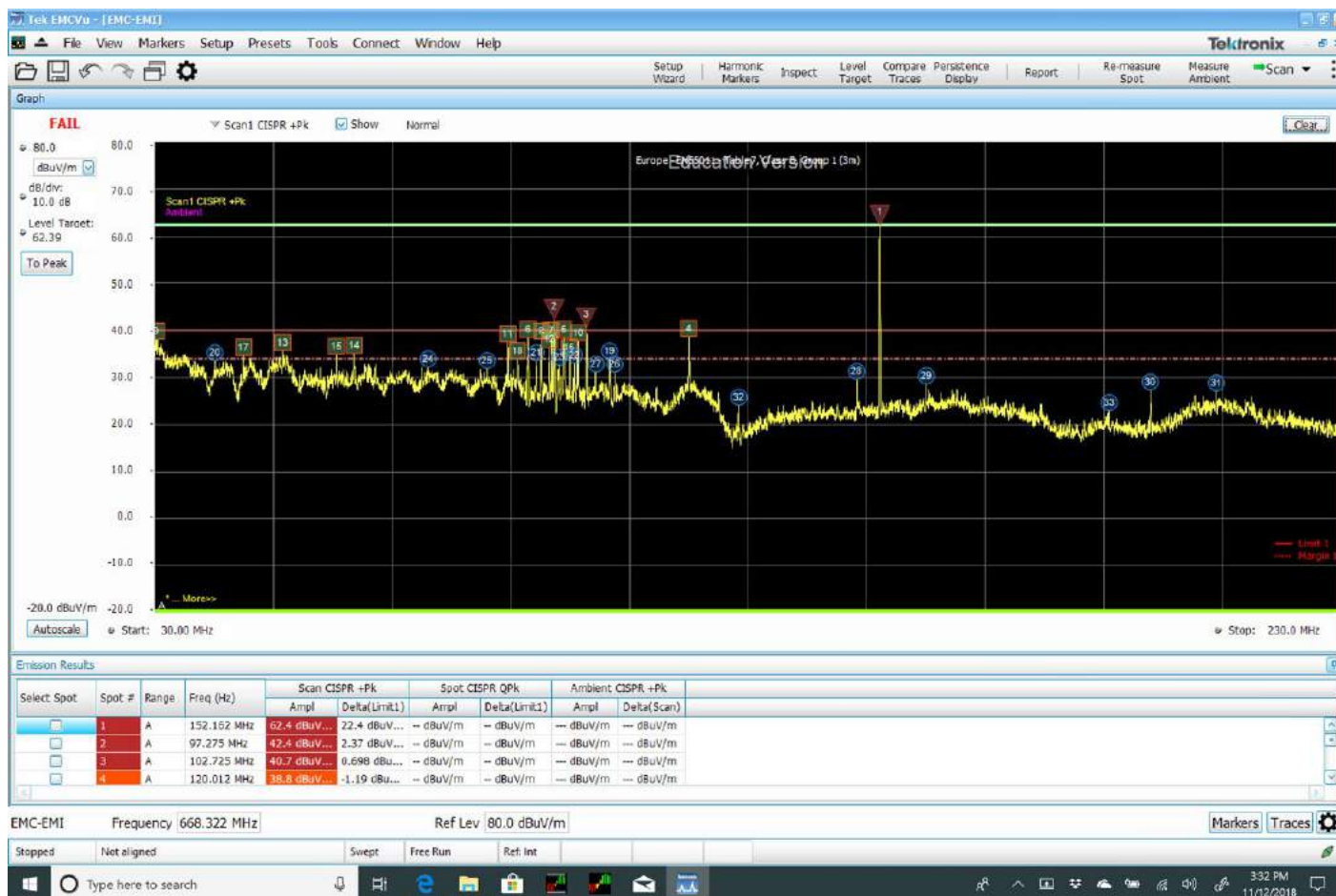
FIGURE 12. Using the Level Target reference (green line) during troubleshooting to tell at a glance whether you're making progress, or not, during implementation of fixes.
