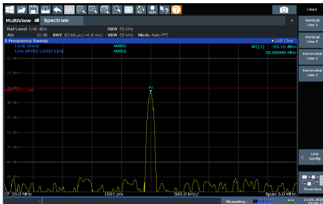
Figure 11-10: Margin violation for limit check
