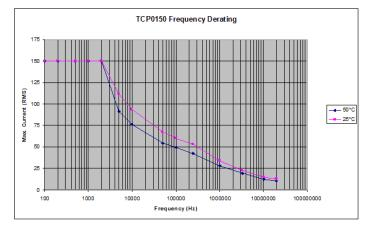
Do not apply currents greater than the max continuous current for more than 10 seconds to minimize heating effects.
