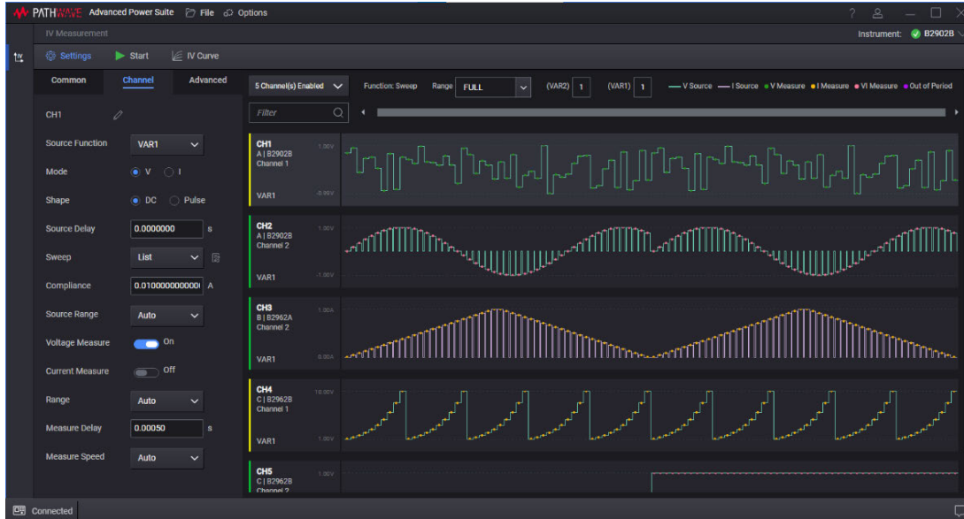
Figure 1. Previewing the settings of multiple SMU channels
