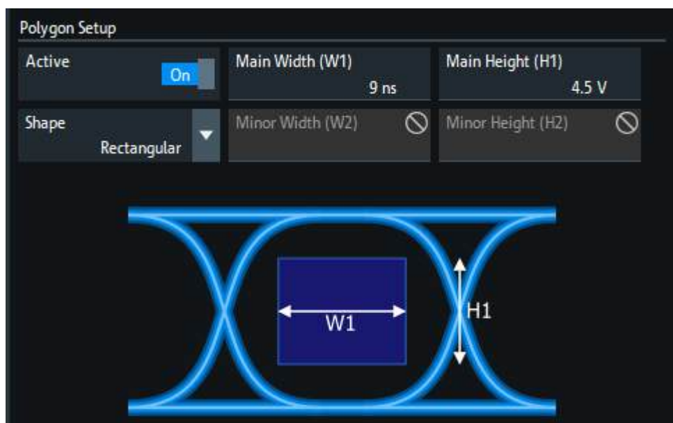
Figure 5-16: Center polygon setup: rectangle
