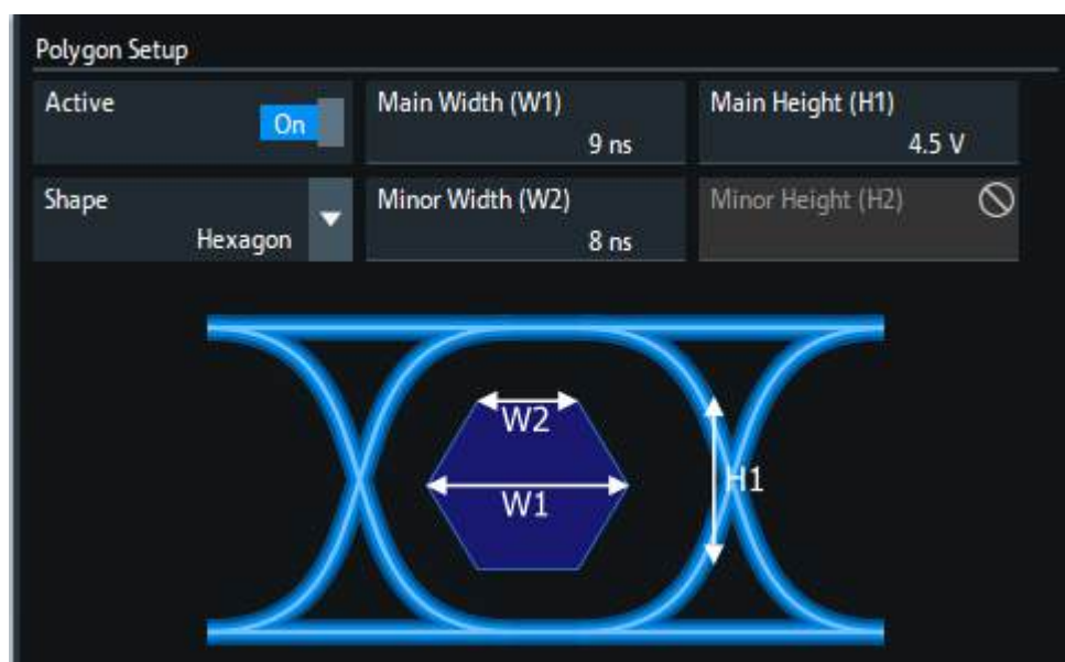
Figure 5-15: Center polygon setup: hexagon
