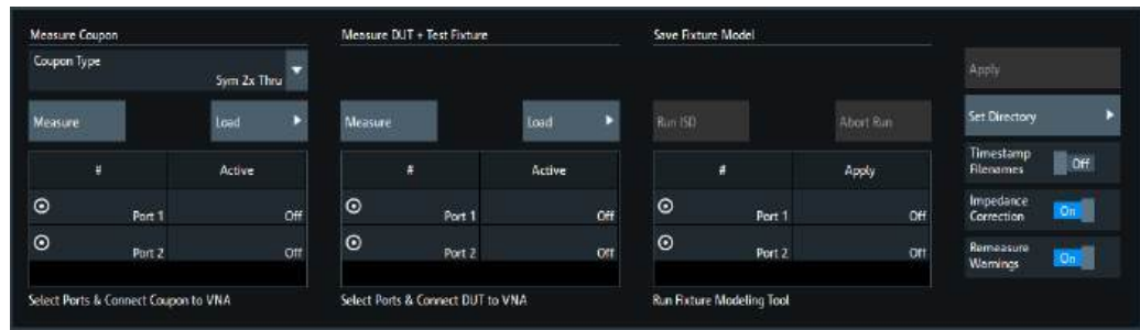
Figure 5-77: Fixture modeling dock widget: single-ended (ISD/SFD/EZD)
