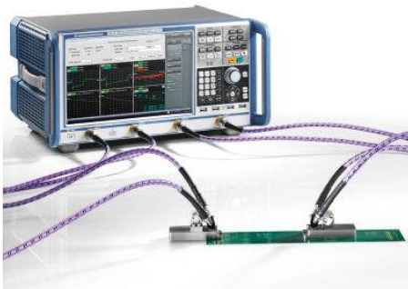
Figure 4-14: Test setup for fixture deembedding
