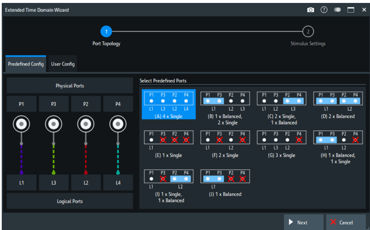
Figure 5-8: Port Topology step ( \leq 4 physical ports)
