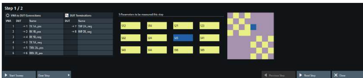
Figure 4-40: Step 3: Measure and/or import S-parameter data
