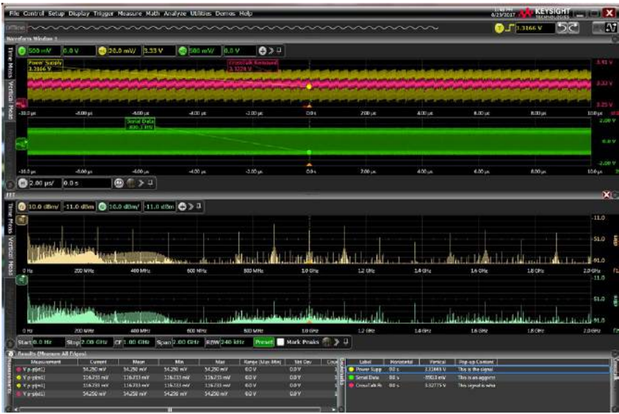
Figure 30. Output from the D9010POWA PI application showing a reduction in the noise on the 3.3 V supply after the effects of the switching loads were removed.
