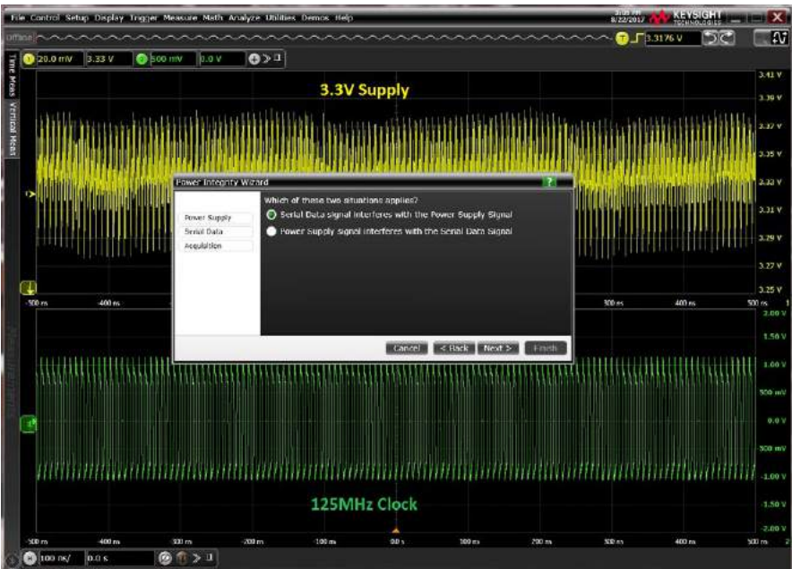
Figure 29. The clock of the digital was probed and is being analyzed as the aggressor to the power rail as shown in the PI setup wizard dialogue (next page).
