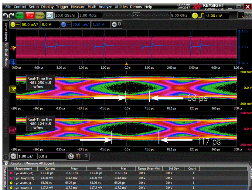
Figure 26. Results from the D9010POWA PI analysis application showing the eye diagram of the FPGA serial data before and after the effects of the DC supply noise are removed. Notice that the results are nearly identical to the previous results where the supply was physically change to
