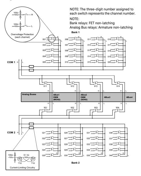
34925A D-Sub Connectors for Two- or Four-Wire Mode
