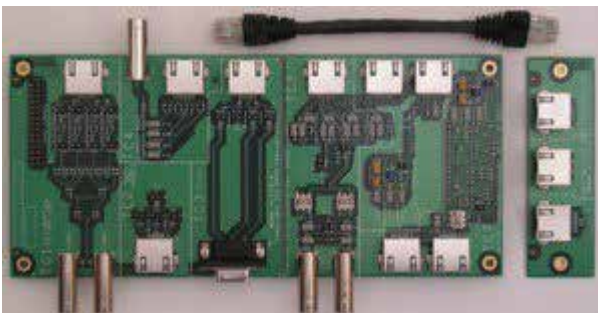
TF-GBE-BTP Basic Ethernet Test Fixture.
