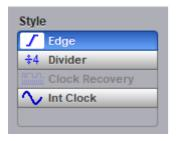
There are several different styles of trigger used in digitizing oscilloscopes. The PicoScope 9400 Series uses **Edge**, **Divided**, **Clock recovery**, **Internal clock** and **External Prescaler** styles.
