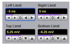
The **Left Limit**, **Right Limit**, **Top Limit** and **Bottom Limit variables** allow you to use the histogram limits to select a region of the database.
