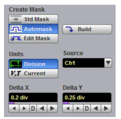
Clicking **Automask** opens a menu for using the reference waveform method. An example of the method for a noisy impulse is shown in the figure below.
