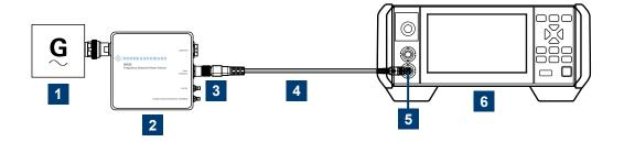
Figure 4-1: Setup with an R&S power sensor (example)
