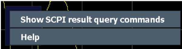
Figure 11-2: Context-sensitive SCPI command menu for a trace in a result display
