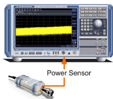
Figure 6-3: Connecting a power sensor using the POWER SENSOR interface
