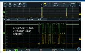
With sufficient memory, the oscilloscope can retain the maximum sample rate (and rated bandwidth) to accurately show the signal. With insufficient memory, the oscilloscope begins reducing the sample rate in order to capture more time. This can lead to insufficient sample rates to accurately show signals.
