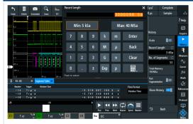
The history and segmented memory offer various user options, providing more flexibility for your applications. Automatic and manual memory configuration are available. In automatic mode, the instrument automatically defines the record length (number of waveform samples that are stored) and the number of history segments. In manual mode, you can set these parameters yourself.
