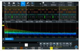
In history mode, all acquisitions can be analyzed at a later time. Individual marked segments can be selected in the acquisition table for display. In addition, the history function can be used to automatically play back all segments. All measurement tools, including the QuickMeas function, mask tests, protocol decoding and FFT are available to analyze the faulty segment.
