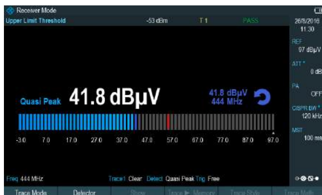
Measurement using quasi-peak detectors with the R&S®FPH-K43 receiver mode option
