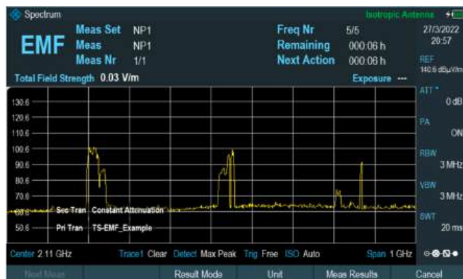
Frequency selective measurement with the R&S®FPH-K105 EMF measurement application option
