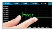
Capture the current drain from all the operating states – sleep mode to active transmit mode – of a component or a product with the DMM7510's digitizing function. Focus in on characteristics of the wave shapes with the touchscreen pinch and zoom features.
