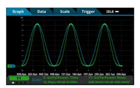
The built-in graphing utility supports displaying and comparing measurements or waveforms from up to four reading buffers at once.
