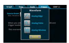
Advanced triggering options make it possible to capture a signal at precisely the right point.
