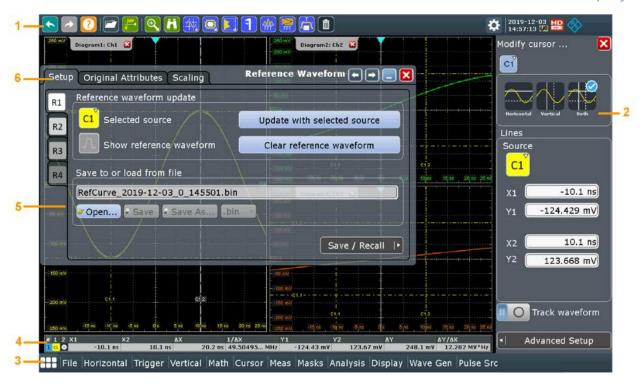
Figure 7-4: Control elements on the touchscreen
