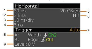
Figure 7-2: Horizontal and trigger label on top of the sidebar
