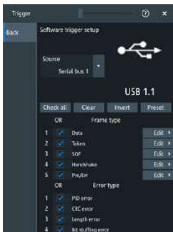
Figure 14-63: Serial bus Software trigger setup dialog for USB 1.1
