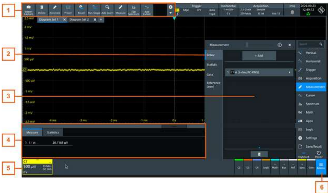
Figure 4-5: Control elements on the graphical user interface
