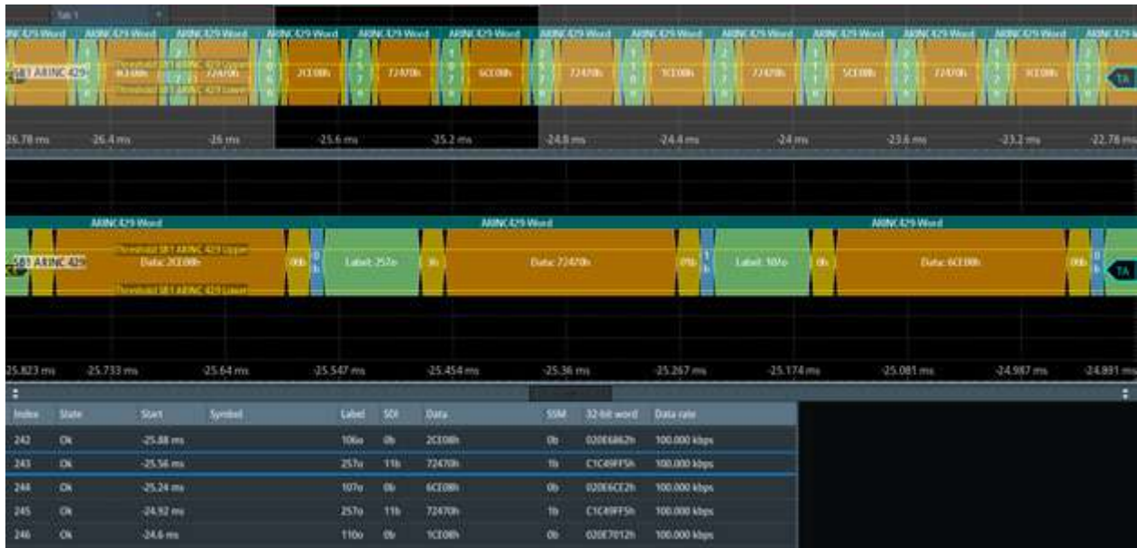
Figure 14-38: Decoded ARINC429 signal
