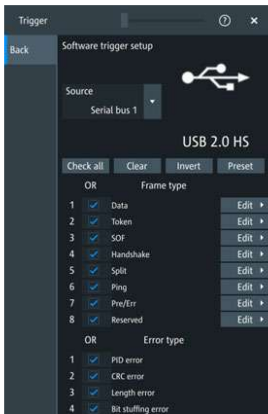
Figure 14-69: Serial bus Software trigger setup dialog for USB 2.0
