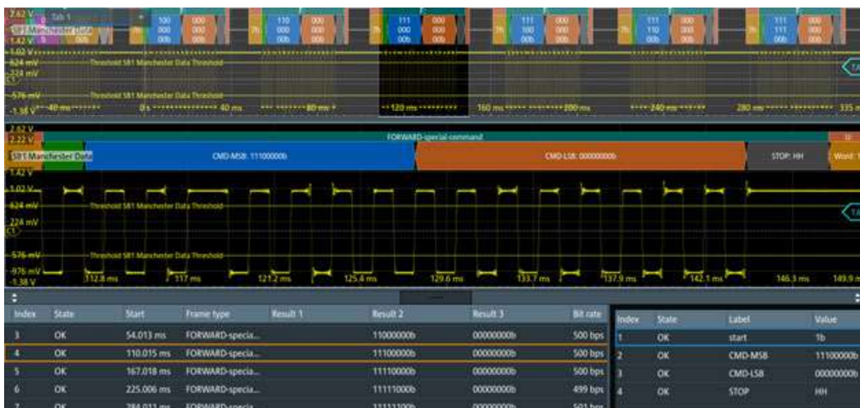
Figure 14-27: Decoded Manchester signal
