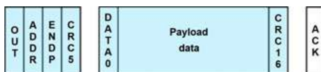
Figure 14-57: Example of a bulk OUT transfer. Blue: host speaks, white: device speaks
