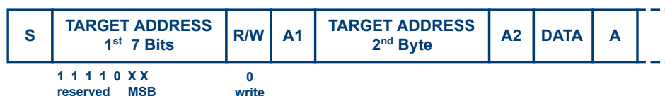
Figure 14-12: 10-bit address, write access
