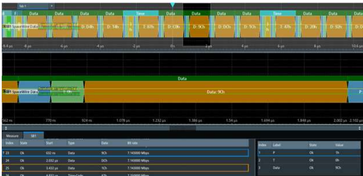
Figure 14-42: Decoded SpaceWire signal
