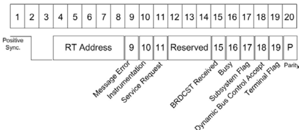
Figure 14-45: Structure of a status word
