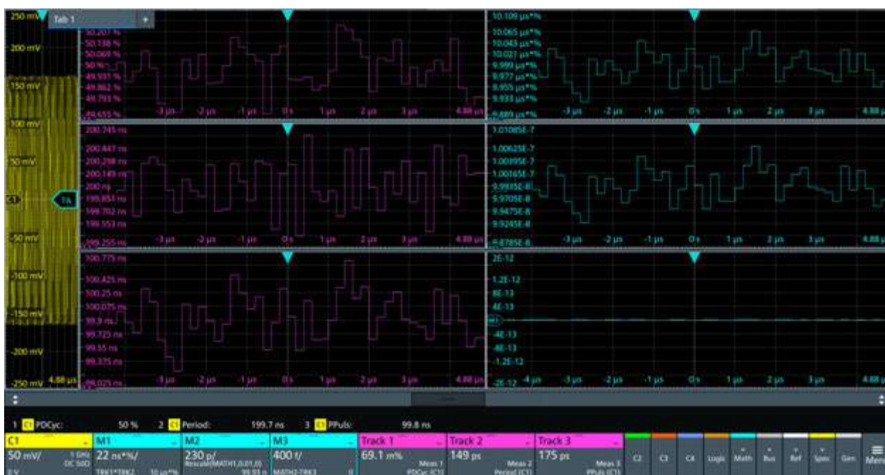
Figure 10-11: Tracks used in math functions
