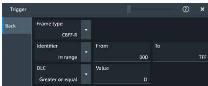
Figure 14-29: Settings for CBFF-R and CEFF-R frames
