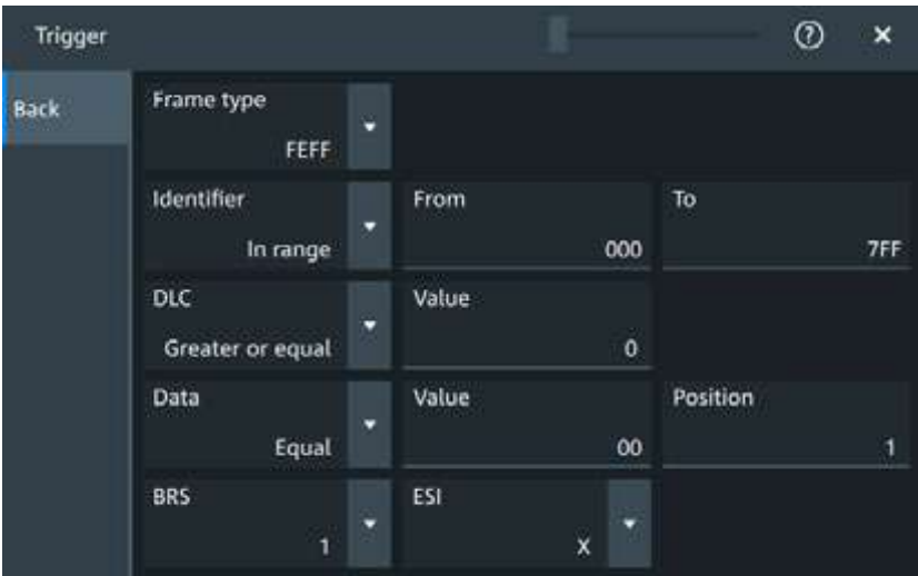
Figure 14-30: Settings for FBFF and FEFF frames
