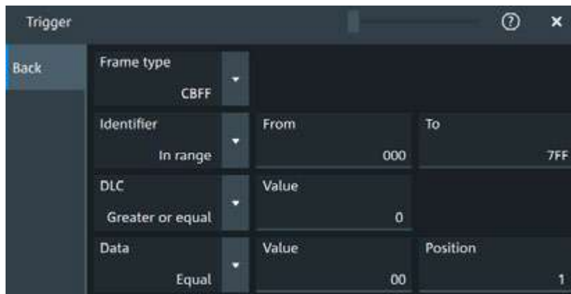
Figure 14-28: Settings for CBFF and CEFF frames
