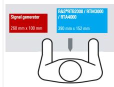
With a depth of less than 16 cm and a weight of only 2.5 kg to 3.3 kg, the R&S\*RTB2000, R&S\*RTM3000 and R&S\*RTA4000 have a compact and handy format. With the R&S\*RTx-B1 arbitrary waveform and 4 bit pattern generator option installed, even more space is saved as the instrument offers the functionality of an entry level signal generator in a single instrument. The small footprint leaves plenty of space on the workbench.
